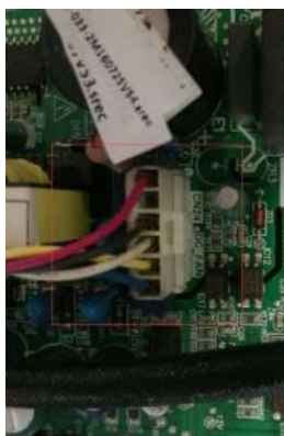
Figure 5.1: Fan connection wiring on indoor unit main PCBs
