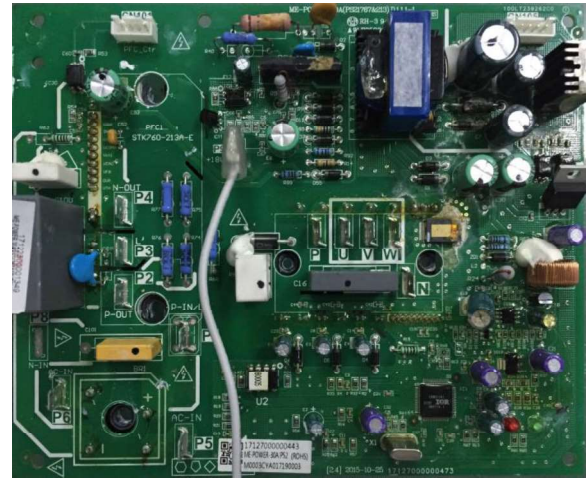
Figure 3-1.2: BCSF030-050 inverter module
